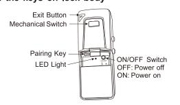
1.Mechanical Switch: Used for installation and equipment trouble, please don't press it often in the normal condition. When press the Mechanical Switch, the lock will be unlocked all the time until open
